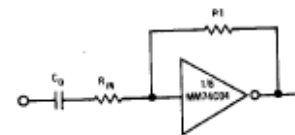
FIGURE 2. A 74CMOS Inverter Biased for Linear Mode Operation.
